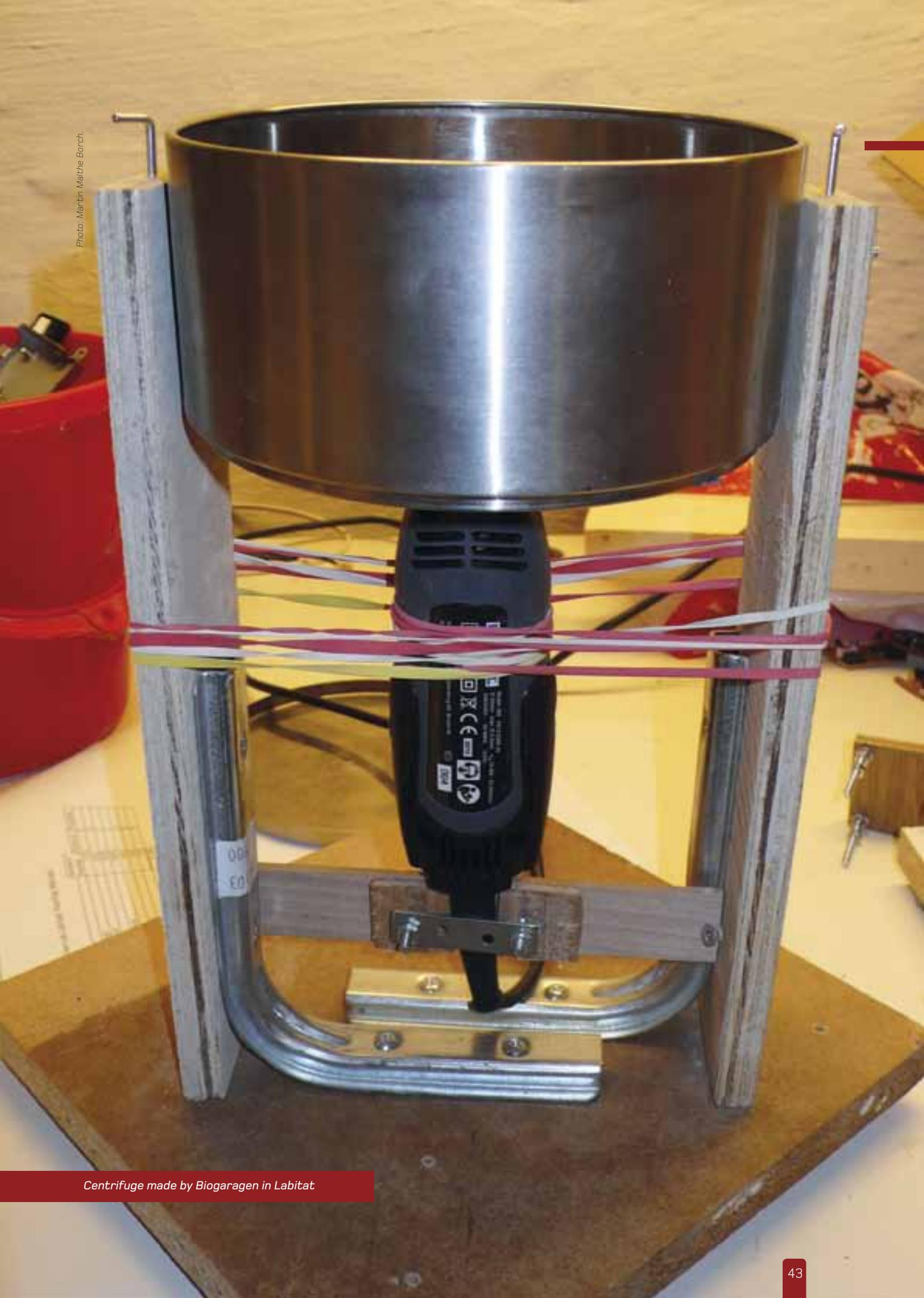
Centrifuge made by Biogaragen in Labitat
